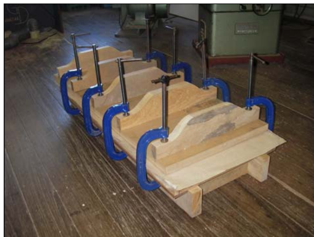
My gluing press - 35 mm MDF with timber frame
