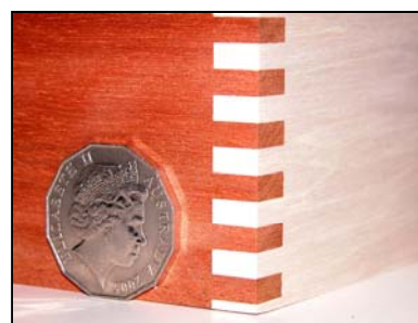
5 mm finger joint in 10 mm timber
