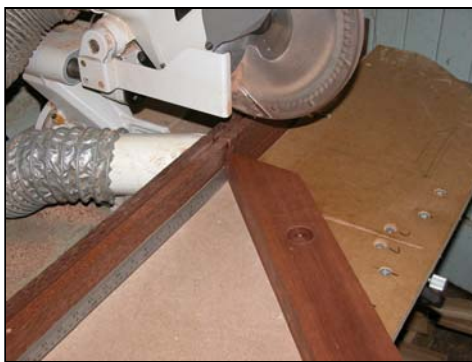
Cutting mitre on 80 x 80 block
