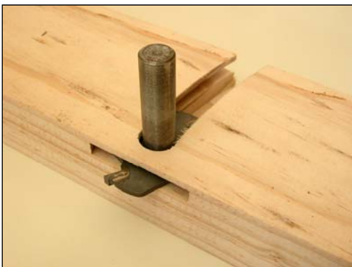
Slot cutter located loosely into fence. Photo shows fence upside down, with face towards camera.
