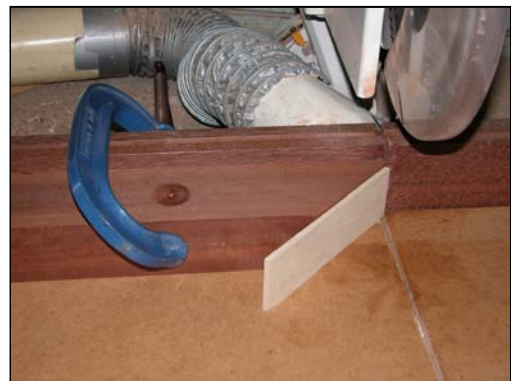
Mitre block in use Hold firmly with one hand while cutting
