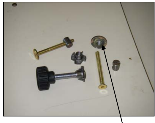
Tee nut inserted into underside of table, along with the range of hardware used.
