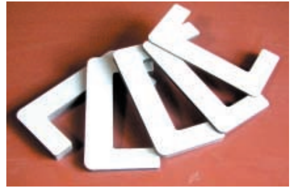
Photo.5: The accessory spacers used to create the variable spacing between pins with the new templates.
