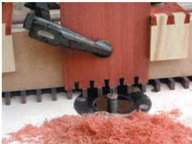
Photo.2: Cutting dovetails with the H10 template.
