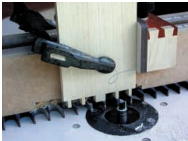
Photo.6: Cutting uneven spaces.
