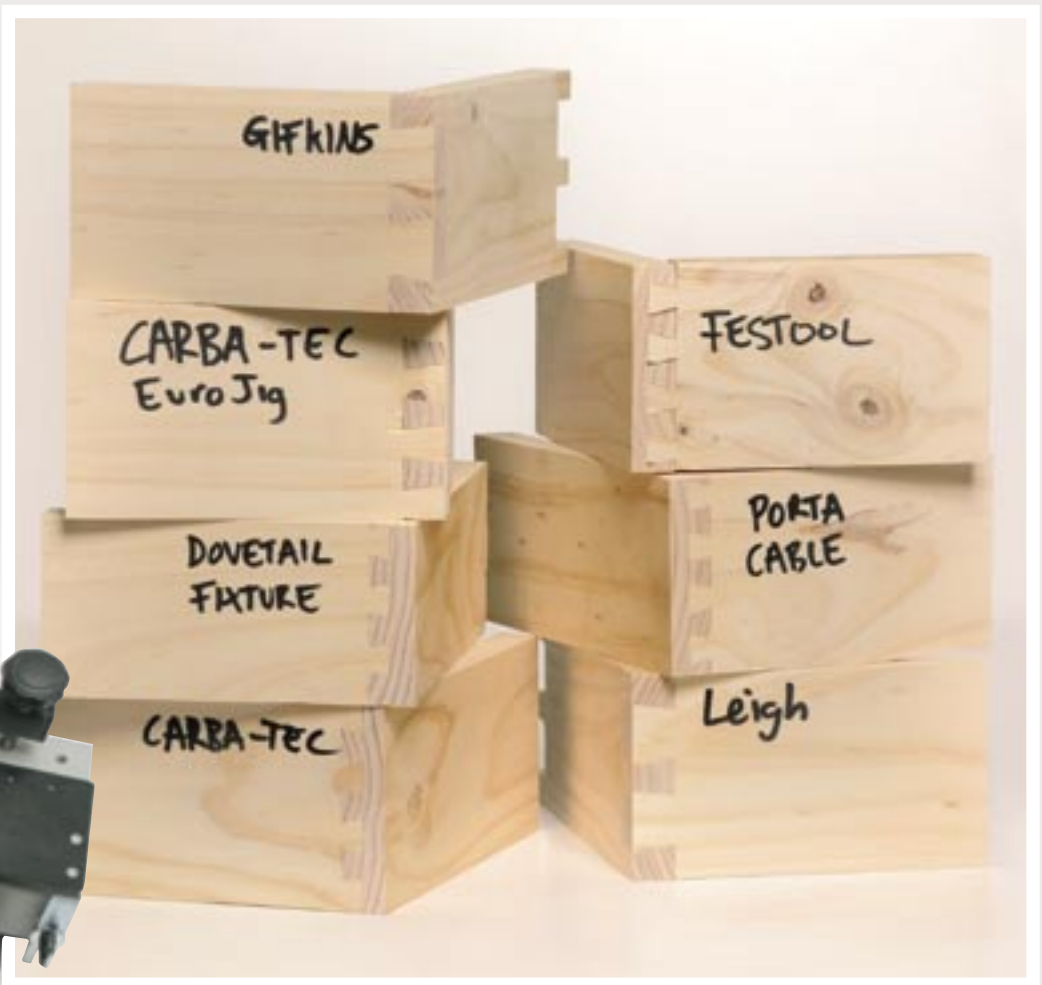
1. Leigh, 2. Euro jig, 3. Carba-Tec WDV-IN, 4. Porter Cable, 5. Gifkins, 6. Sherwood Dovetail Fixture, 7. Festool.
