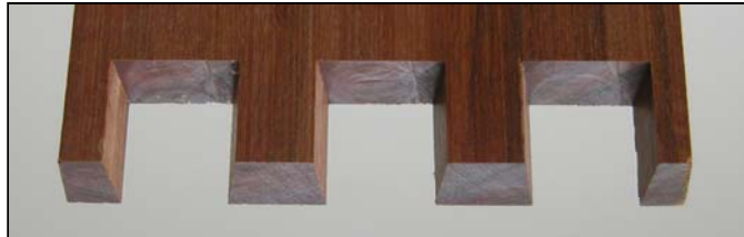
Pins are cut on the tapered fingers with a straight cutter.
