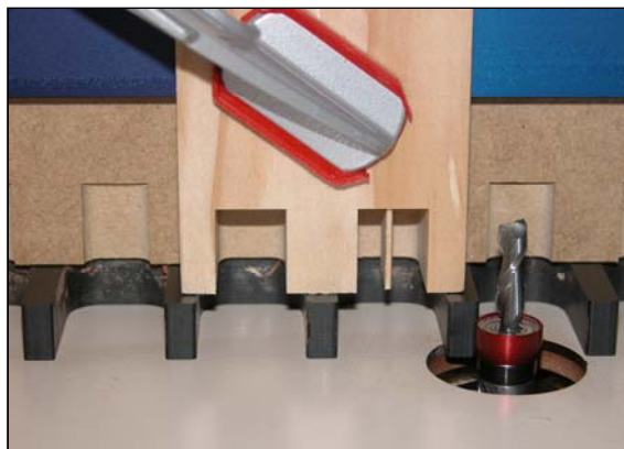
Waste not fully removed in right hand cut
