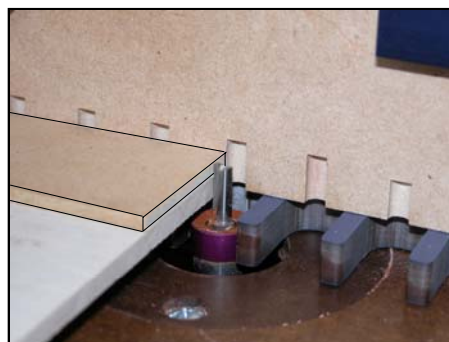
Set height of cutter to thickness of workpiece plus spacer plus template
