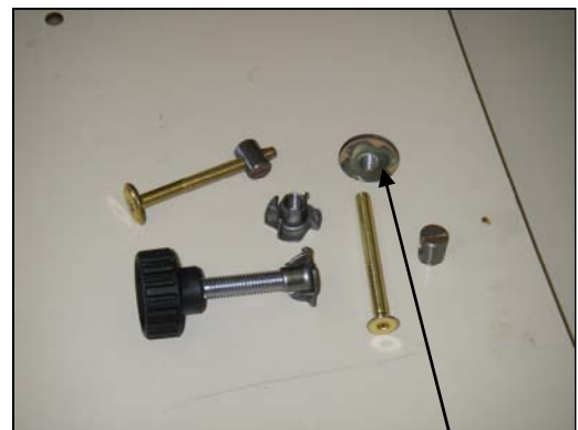
Tee nut inserted into underside of table, along with the range of hardware used.
