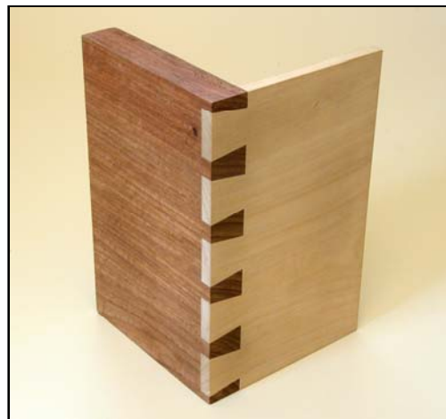
Dovetail joint in 22 mm and 8 mm timber, cut on the B10 template
