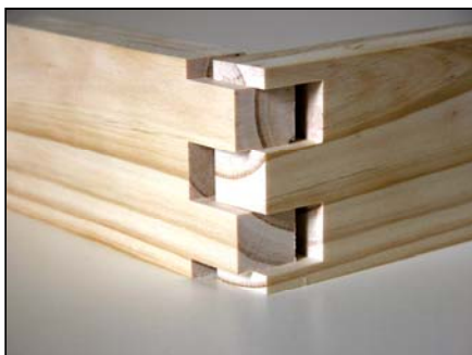
Photo: 55 mm board with 5 mm fingers top and bottom cut on the F15 template
