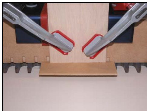
3 mm workpiece with 3 mm spacer under workpiece on the F5 template
