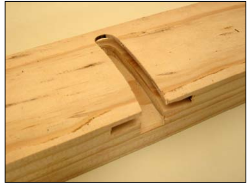
Fence for slot cutter. Photo shows fence upside down, with face away from camera.
