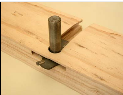
Slot cutter located loosely into fence. Photo shows fence upside down, with face towards camera.
